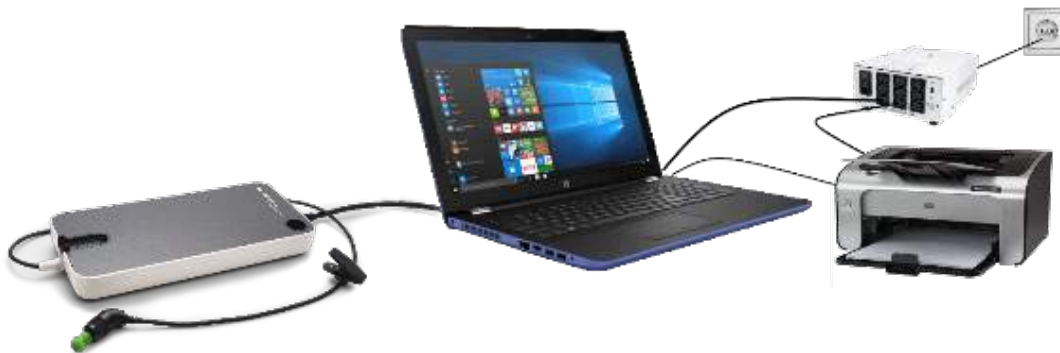
Fig. 2. Lyra connected to the PC/Laptop connected to a medical approved transformer.
