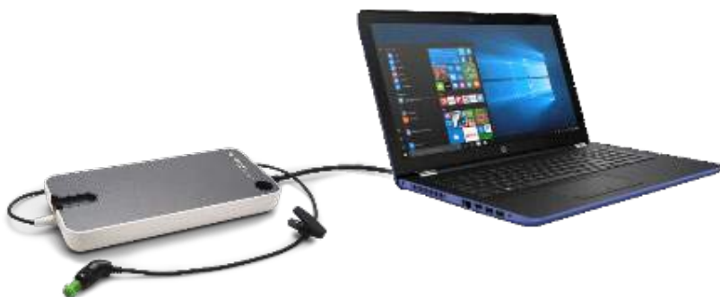
Fig. 2. Lyra connected to the PC/Laptop connected to a medical approved transformer.
